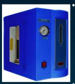
*HGH-300 and HGH-500* high purity hydrogen generators are based on the technology of astronautic fuel cells, in which hydrogen is produced by the electrolysis of water, and the produced oxygen is released into the atmosphere.
