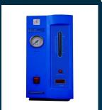
HGN-300 & HGN-500 nitrogen gas generators utilize theories of physical adsorption and electrochemical seperation and use rare metal as catalytic agent. The instrument can directly extract highly pure (as high as 99.999%) nitrogen from the air. There is no need of deoxidation. The generators are compact and advanced in technology. They are very suitable for gas chromatographs and micro coulomb meters.
